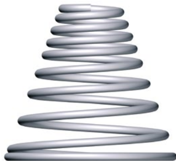
7. Conical compression spring gives a progressive spring characteristic
